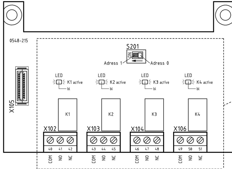
⚠ Contact load in case of 30VDC: 5A ohmic
