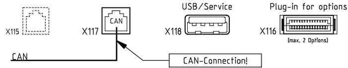
Only for version "Inversed" with optional fire-protection PCB
