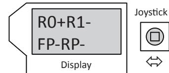
3. Enabling of the desired function per relay: under Settings ⇒ Configuration RC0.1 up to RC0.4 (for Addr 0) and RC1.1 up to RC1.4 (for Addr 1).
