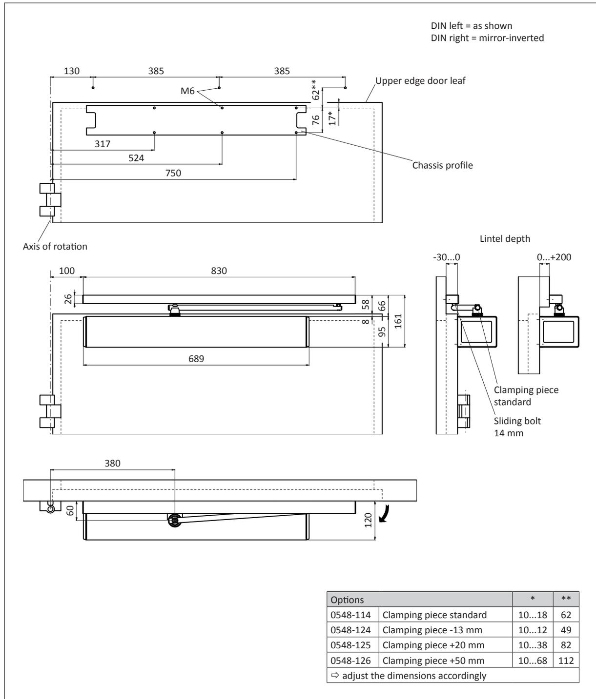
2. Mount the drive mechanism.
